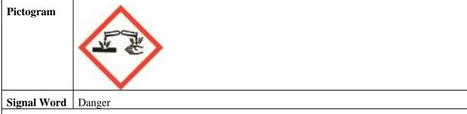
**Hazard Statements:** May be corrosive to metals (H290), Causes severe skin burns and eye damage (H314).
