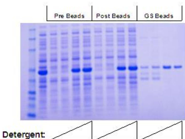
Figure 2 – Solubilization and Renaturation of GST-RTK fusion protein. GST-RTK expression was induced with 1 mM IPTG at 37°C for 4 hrs. Cell pellet was lysed, and inclusion body was solubilized and renatured under different amounts of detergent solubilization solution according to the assay protocol. Lane 1: MW STD; Lane 2: Whole E.Coli lysate; Lane 3, 7, 11: No detergent; Lane 4, 8, 12: 32-fold dilution; Lane 5, 9, 13: 8-fold dilution; Lane 6, 10, 14: 2-fold dilution.
