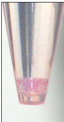
Figure 1: RalBP1 PBD Agarose beads, in color, are easy to visualize, minimizing potential loss during washes and aspirations.
